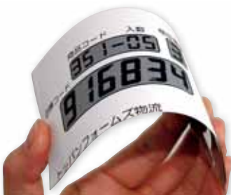
Electronic paper labels have a paper-like thickness of just 0.4mm and enable barcodes and other displays to be rewritten using radio-frequency transmission.
