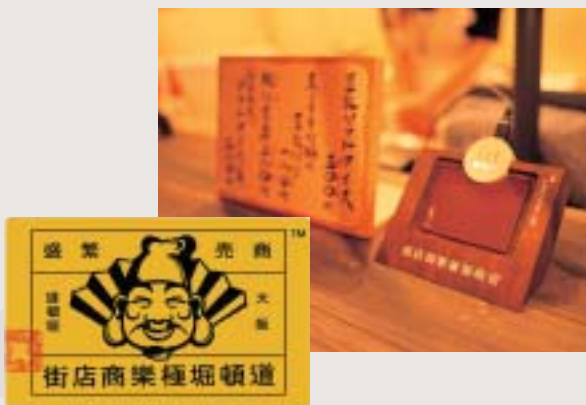
This payment system, which uses contactless IC cards, has been installed in a theme park in Japan.
